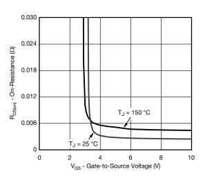
On-Resistance vs. Gate-to-Source Voltage
