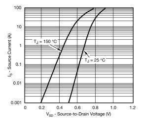
**Source Drain Diode Forward Voltage**
