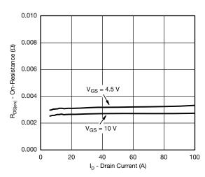
On-Resistance vs. Drain Current
