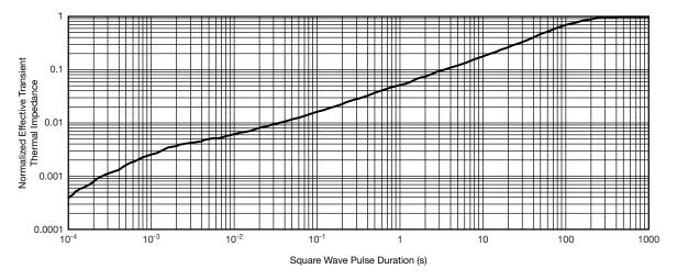
Normalized Thermal Transient Impedance, Junction-to-Ambient
