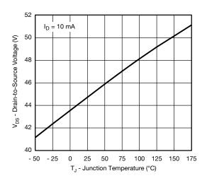
**Drain Source Breakdown vs. Junction Temperature**
