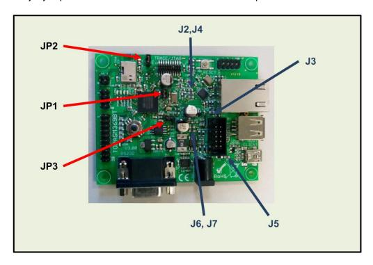
The jumpers JP1 and JP2 are normally closed. They can be opened to separate the microcontroller or the Bluetooth® module from VCC and to insert an ammeter there in order to measure current draw.
