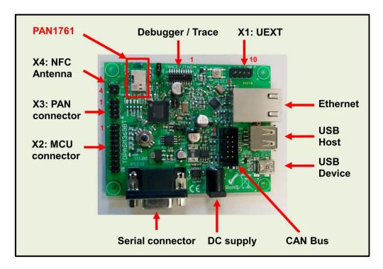
The board is generic and other starter kit use different type of modules. This board is equipped with PAN1761.
