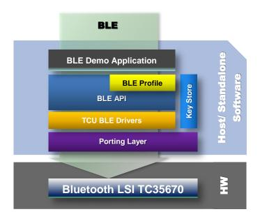
The easy to use high-level BLE API for PAN1761 shown above helps to setup, connect and to transfer data in an easy way. Driver layer provide access to the entire function set of the module. Bluetooth® Low Energy application example is available on Toshiba CortexM3 MCU with FreeRTOS integration.
