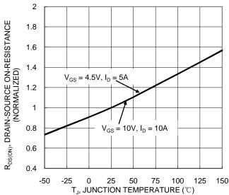
Figure 6. On-Resistance Variation with Temperature
