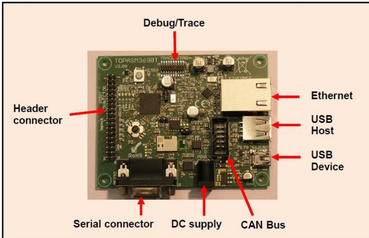
The board can be powered in three ways:
