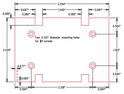
1. PCB is symmetrical in the X and Y directions.
