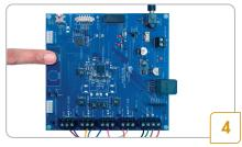
Touch the ON/OFF CapSense® button to toggle the LEDs. Touch the COLOR CapSense button to cycle through colors
