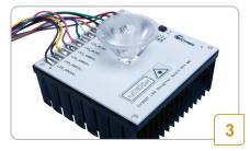
Mount the optical diffuser on the LED daughter board. Connect the power supply to the main board
