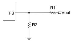
Figure 3 Feedback Divider Network
