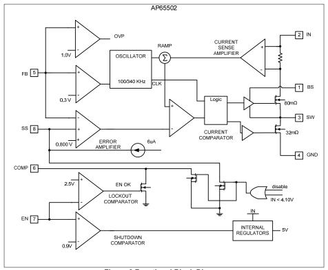
Figure 2 Functional Block Diagram
