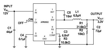
Figure 1 Typical Application Circuit
